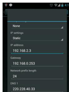
Go to **Settings - Wi-Fi - press & hold Selected SSID to modify network - then click on Show advanced options.** Click **IP settings** to choose **Static** to enter address such as **192.168.2.XXX** (XXX can be set from 1-128)
