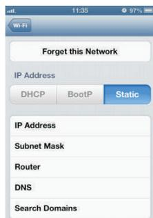
Go to **Settings - Wi-Fi - Selected SSID - advanced settings**, then click on **Static** to enter IP address such as **192.168.2.XXX** (XXX can be set from 1-128) and Subnet Mask **55.255.255.0**
