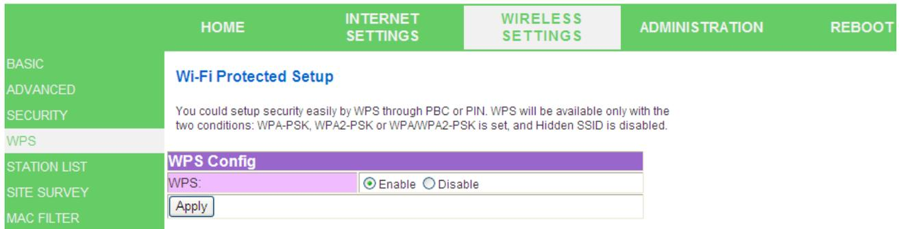
This function helps to establish the Wi-Fi security. For AP mode, it can be setup one WPS method including PIN (Personal Identification Number) and PBC (Push Button Certification).
